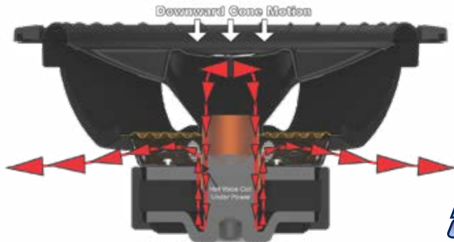
As Cone Moves Downward, Hot Air from Voice Coil is Forced out of the Woofer.
